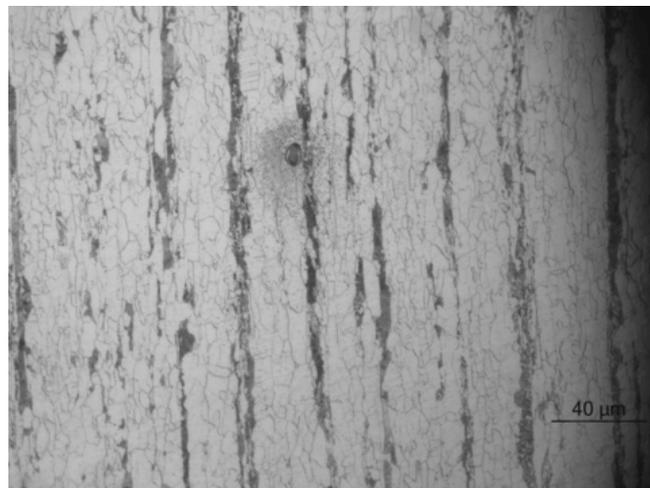
FIGURE 69: Microstructure X70 brut 2
