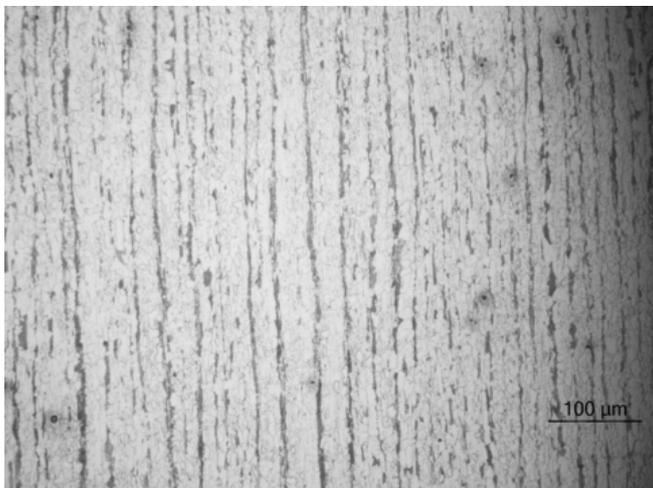
FIGURE 68: Microstructure X70 brut 1
